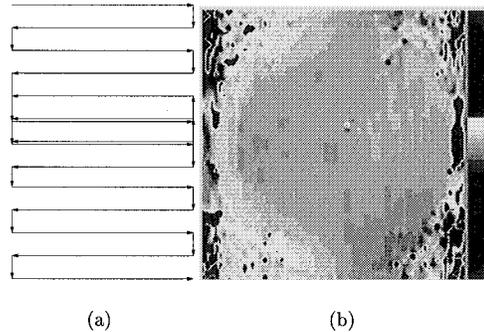
Figure 1: (a)  $K$ -space trajectory used for real-time magnetic field mapping, and (b) resulting field map (full scale is -4.2 ppm to +4.2 ppm)
